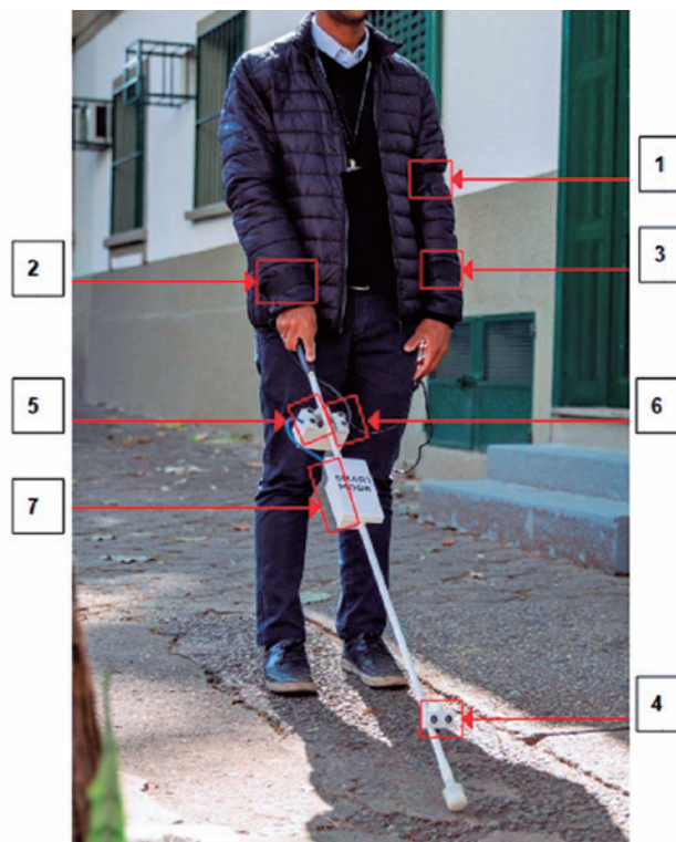
Source: Alex Reipert (Photographer; Universidade Federal de São Paulo). Note: (1) Wristband A notifies the presence of obstacles on the ground. (2) Wristband B notifies the presence of obstacles higher to the right. (3) Wristband C notifies the presence of obstacles higher to the left. (4) Sensor A detects obstacles on the ground. (5) Sensor B detects obstacles higher to the right. (6) Sensor C detects obstacles higher to the left. (7) Portable power bank (20) .
