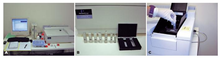
**Figure 1.** A) Spectrophotometer Perkin Elmer Lambda 35 UV/VIS used in this experiment. B) Different lens holders designed and built especially for placing the sample in the spectrophotometer. The three holders on the left are the holders for the pig lenses. C) Placement of lens holder with the crystalline lens directly in front and covering the complete entrance hole of the integrating sphere of the spectrophotometer.
