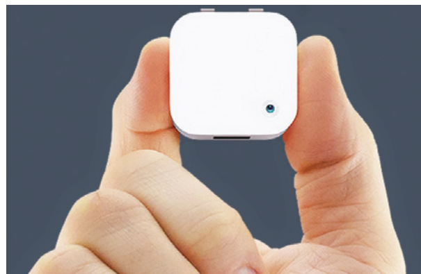
Figure 1. Narrative Clip camera. The image shows the Narrative Clip camera held by an adult hand for size reference. Features: dimensions, 36 × 36 × 9 mm; weight, 20 g; capacity, 6000 photographs; image-capture frequency, 30 s; resolution, 5 megapixels; battery life, 2 days.
